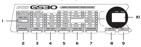
**Comp/Wah** - This button will access the Compressor and Wah effects. Successive presses of this button ill toggle between the Compressor and the Wah. The selected effect is indicated by the flashing LED. The status f the selected effect can then be changed by rotating the Data Wheel. Compression and Wah can be used multaneously. See page 19 for a complete description of Compression and Wah effects.
